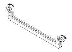
**4.** Paying attention to the location of the notch on the memory module and the orientation, insert it vertically within the guides at either side of the socket.
